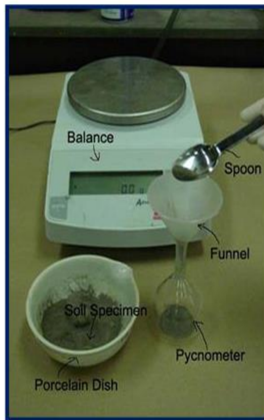
Figure. 3-1 Equipment and tools for Specific Gravity test
