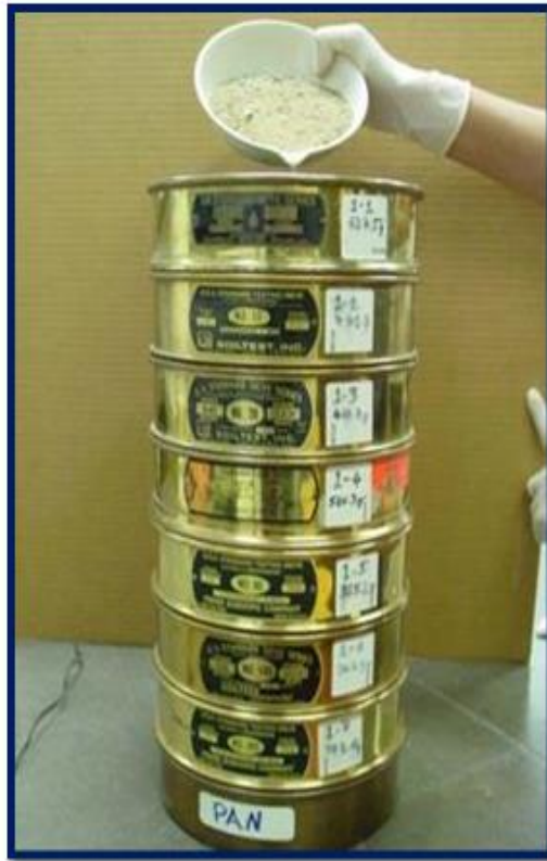
Figure 4-1. A stack of sieves with a pan at the bottom and a cover on the top.
