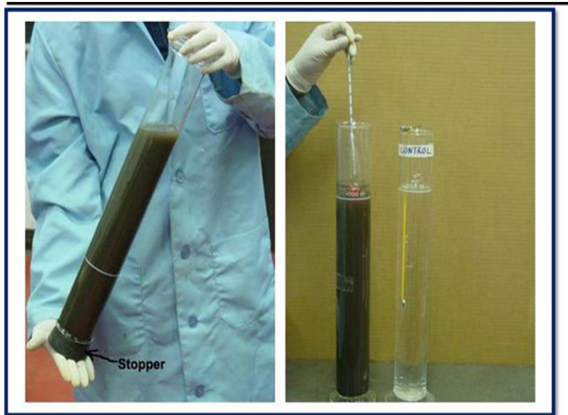
Figure 5-2. Equipment for hydrometer test.
