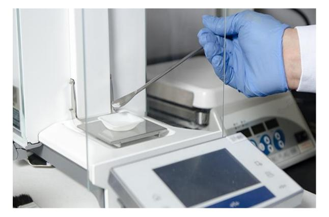
5- Place the container with the substance back on the balance platform if necessary and record the mass as indicated by the digital display. Then you must press (OFF) button to shut down the device.
