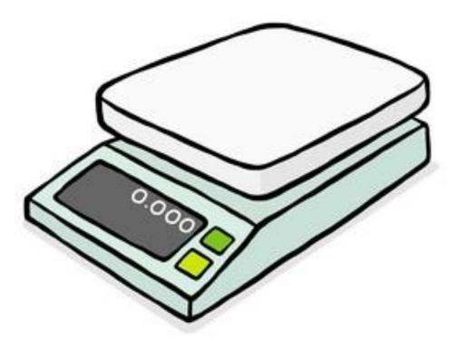
2- clean the surface of the balance before using because Fingerprints and other greases from your hands add mass and must be avoided for accurate measurements. , then Press the "ON" button and wait for the balance to show zeroes on the digital screen.
