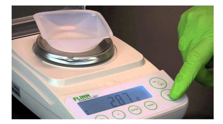
4- Press the "Tare" or "Zero" button to automatically deduct the weight of the container from future calculations. The digital display will show zero again, indicating that the container's mass is stored in the balance's memory.
