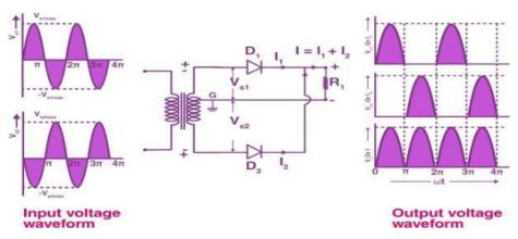
The circuit of the full wave rectifier consists of a step-down transformer and two diodes that are connected and center tapped. The output voltage is obtained across the connected load resistor.
