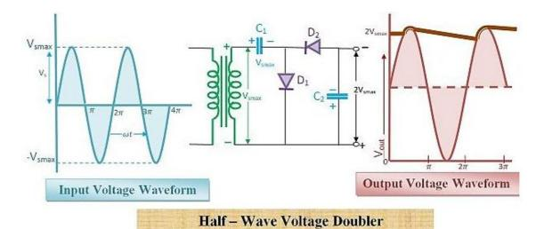
During positive half of AC cycle, the diode D2 is reverse biased thus the diode D2 becomes an open circuit, and the capacitor C2 will remain un charged.
