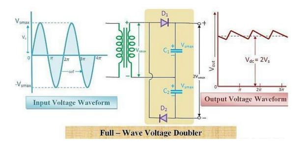
When the negative half cycle of AC is applied to the full wave voltage doubler circuit, the diode D2 will be forward biased. Due to this, the capacitor C2 starts
