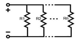
$$R_{\text{total}} = \frac{1}{\frac{1}{R_1} + \frac{1}{R_2} + \frac{1}{R_3} + \dots + \frac{1}{R_n}}$$
