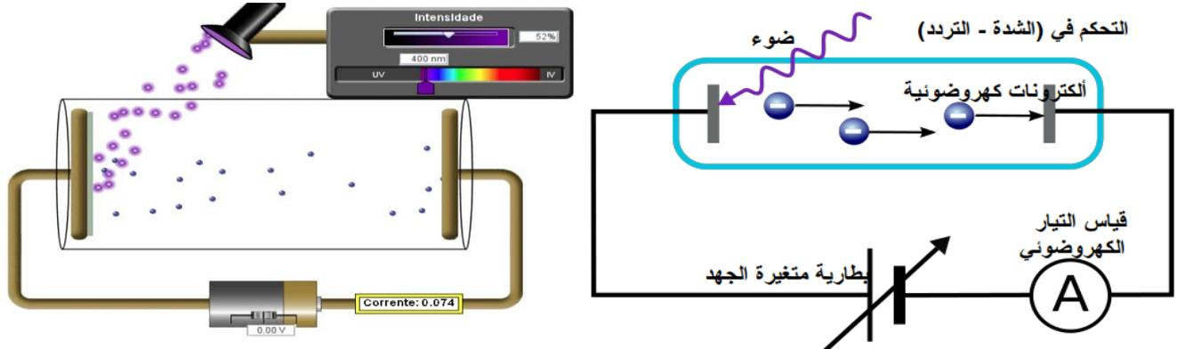
Figure 1 (The working principle of the photoelectric cell)
