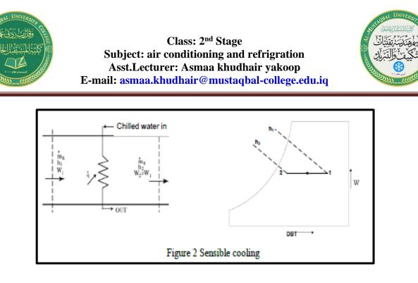
Calculate the cooling load when 1.5 m<sup>3</sup>/s of moist-air, initially at a state of 21 °C DBT, 15 °C WBT and 101.325kPa barometric pressure, 1 is cooled sensibly by 5 °C using cooler coil, what is the flow rate of chilled water necessary to effect this cooling if the flow return temperature of 10°C and 15 °C satisfactory.
