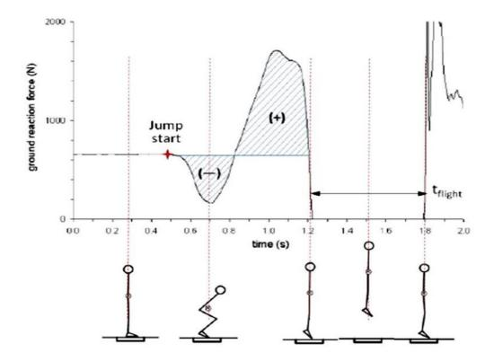
Figure 1: Vertical ground reaction force (Fz) measured by the force plate during a standing vertical jump
