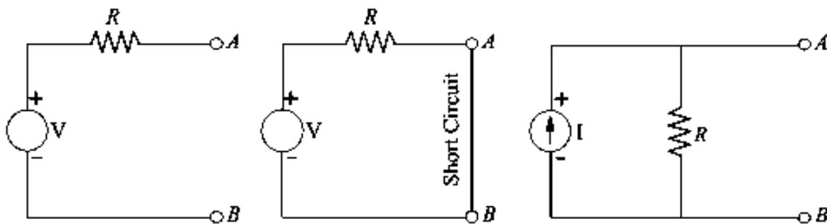
**Example 1:** Convert the voltage source into an equivalent current source.
