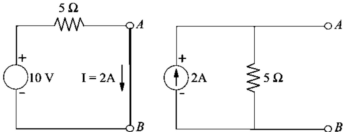
**Example 2:** Find the equivalent voltage source for the current source in the circuit shown below.
