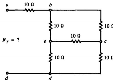
**Solution:** transform the star network into its equivalent delta
