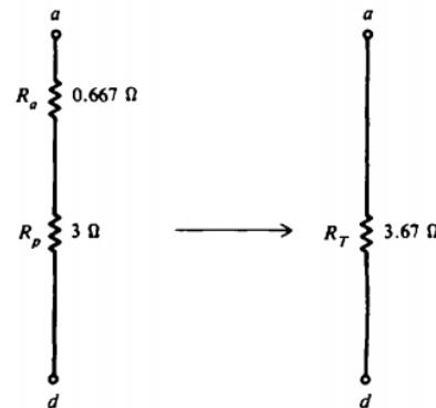
**Example 8:** Reduce the bridge circuit shown below **to** a single equivalent input resistance at terminals **a** and **d**.
