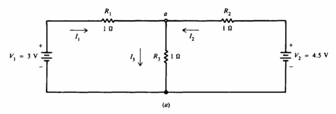
**Solution:** Find the currents produced by voltage source  $V_1$  only. Replace voltage source  $V_2$  with a short circuit
