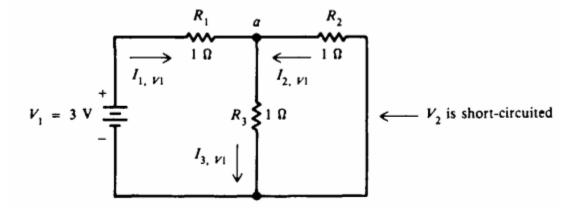
In order to calculate the value of I<sub>1</sub> we find the equivalent resistance
