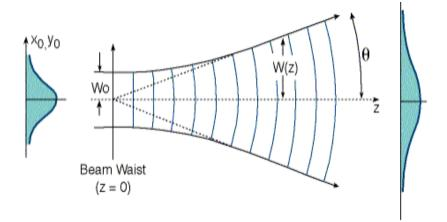
The laser beam is a single-phase Gaussian beam ( $TEM_{00}$ ) that depends on the size of the spot at the waist( $W_0$ ), the spot size at the distance from the waist (W) can be written as follows
