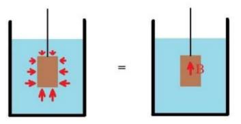
Where  $(\rho)$  is the density of the fluid, V is the volume of fluid displaced and g is acceleration due to gravity. It is the buoyant force that keeps ships afloat in water.
