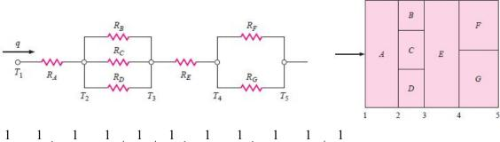
$$\frac{1}{R_{1}} = \frac{1}{R_{A}}; \quad \frac{1}{R_{2}} = \frac{1}{R_{B}} + \frac{1}{R_{C}} + \frac{1}{R_{D}}; \quad \frac{1}{R_{3}} = \frac{1}{R_{E}}; \quad \frac{1}{R_{4}} = \frac{1}{R_{F}} + \frac{1}{R_{G}}$$
