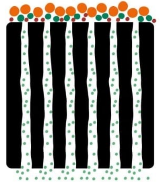
Membrane Filtration: Traps particles larger than pore size
