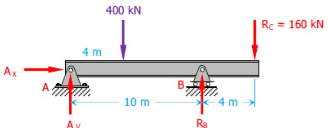
**Example No. 3:** Determine the horizontal and vertical components of reaction on the member at the pin A, and the normal reaction at B in Figure.
