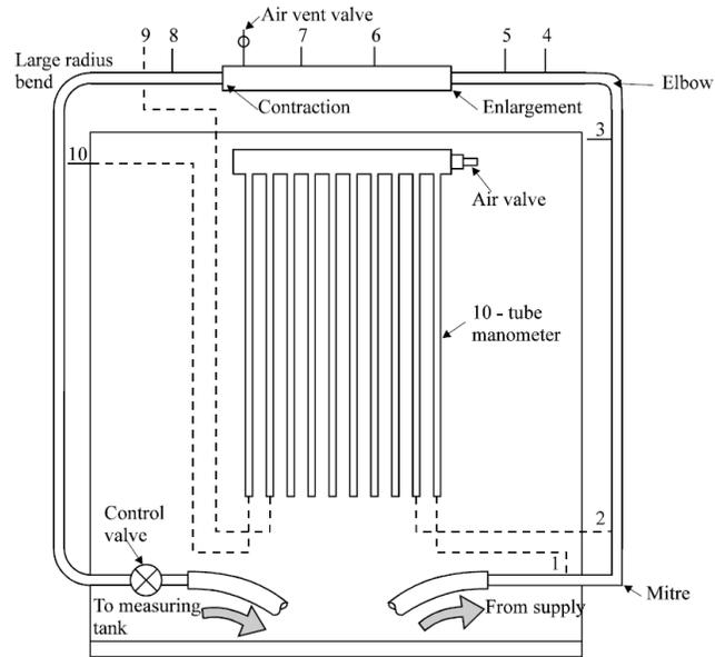
Fig 10.2 Arrangement of apparatus for measuring losses in pipe fittings.
