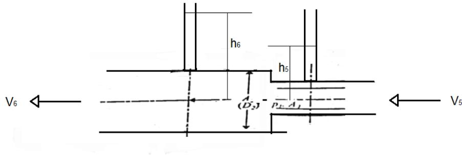
Fig 10.4 Losses in enlargement fitting.
