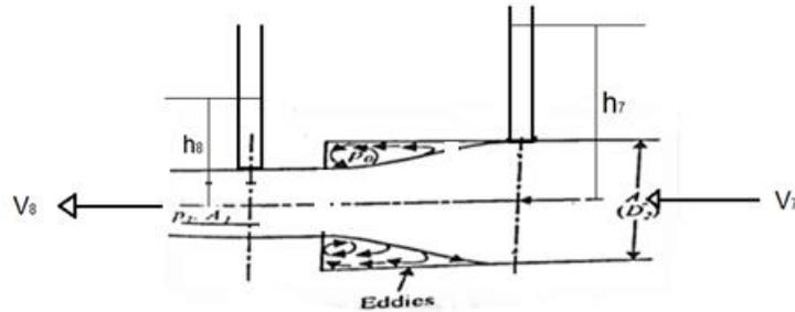
Fig 10.5 Losses in contraction fitting.
