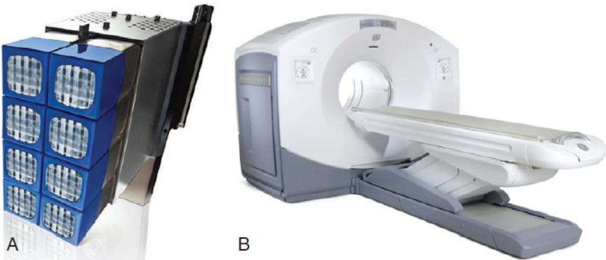
Figure (11):A, Modular cassette from a PET scanner containing eight block detectors. These cassettes are mounted on the PET scanner gantry to form complete rings of detector blocks that surround the patient. B, Clinical PET scanner based on rings of these block detectors.
