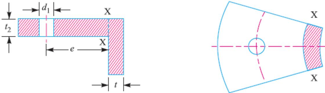
$e = \text{Pitch circle radius} - (\text{Radius of bolt hole} + \text{Thickness of cylinder wall})$
