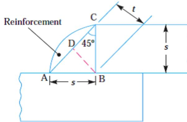
The minimum area of the weld is obtained at the throat  $BD$ , which is given by the product of the throat thickness and length of weld.
