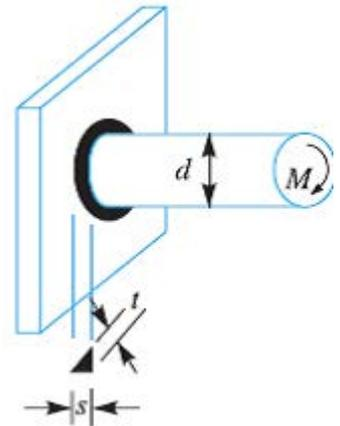
This bending stress occurs in a horizontal plane along a leg of the fillet weld. The maximum bending stress occurs on the throat of the weld which is inclined at  $45^\circ$  to the horizontal plane.
