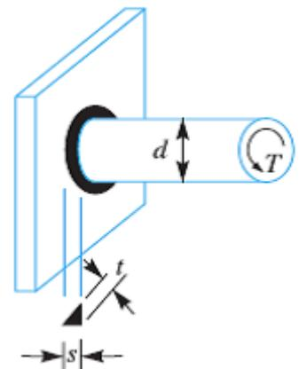
This shear stress occurs in a horizontal plane along a leg of the fillet weld. The maximum shear occurs on the throat of weld which is inclined at  $45^\circ$  to the horizontal plane.
