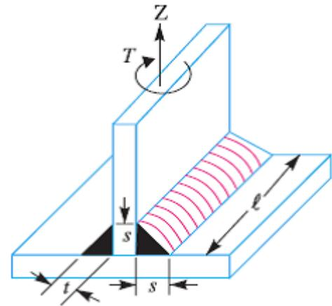
The maximum shear stress occurs at the throat and is given by
