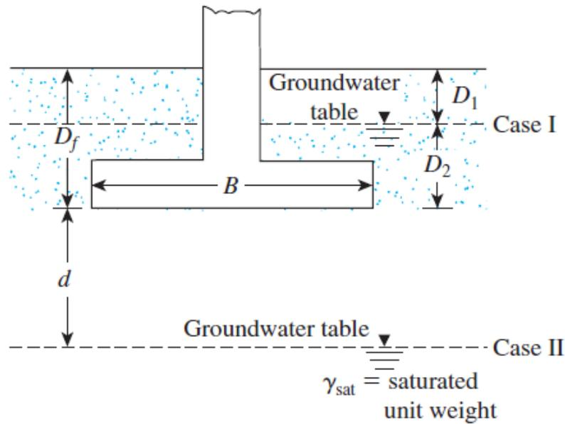
**Case I.** If the water table is located so that  $0 \leq D_1 \leq D_f$  the factor  $q$  in the bearing capacity equations takes the form:
