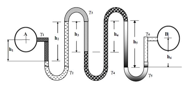
$$P_A + \gamma_1 h_1 - \gamma_2 h_2 + \gamma_3 h_3 - \gamma_4 h_4 + \gamma_5 h_5 - \gamma_6 h_6 = P_B$$
