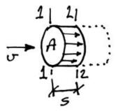
The fluid at 1-1 moves a distance of s = vt to 2-2. Therefore in 1 second it moves a distance of v. The volume moving per second is thus:
