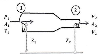
$$\frac{P_1}{\gamma} + \frac{V_1^2}{2g} + Z_1 = \frac{P_2}{\gamma} + \frac{V_2^2}{2g} + Z_2 \dots \underline{\text{Burnoulli's Equation}}$$
