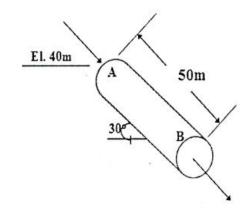
Example 17 Find the discharge of Oil (r.d.=0.85) through the pipeline and the velocity at pint 2 for 55 Kpa pressure at point 1.
