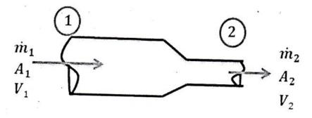
$\dot{m} = \dot{m}_1 = \dot{m}_2 = \text{constant}$ , where  $\dot{m} = \rho VA$  (mass flow rate). Units  $\rightarrow Kg.m^3/s$
