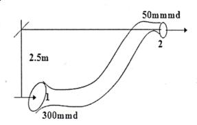
$$V_{1} = \frac{Q}{A_{1}} \qquad V_{2} = \frac{Q}{A_{2}}$$
