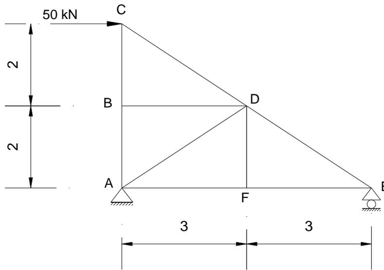
H.W2 : For the simple truss shown in fig. find the axial force in bars AB, AF,AE, BC & CD.
