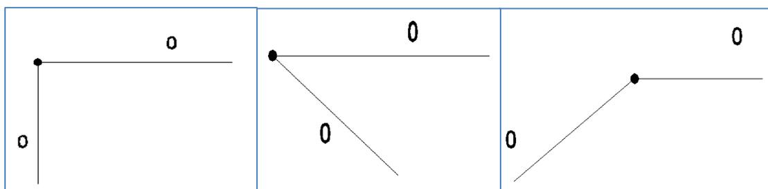
2- When met three bars in joint two of them on one straightness and there is no external force on this joint, we conclude that the force in third bar equal to zero.
