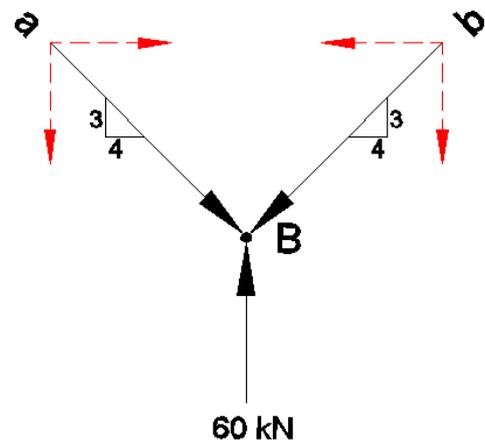
Ex5: For the compound truss shown in fig. find the axial force in bars a, b & c
