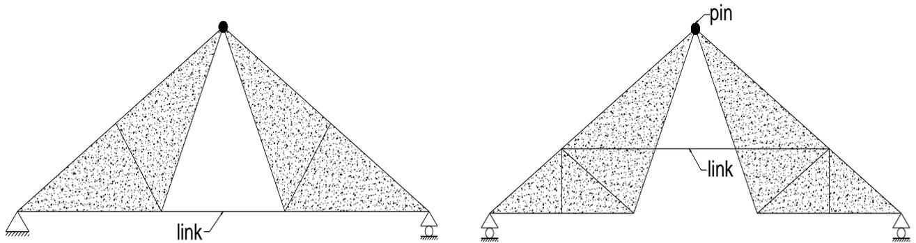
iii- A pin and two links intersecting at support
