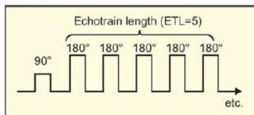
Fig.(2): Schematic illustration of fast spin echo
