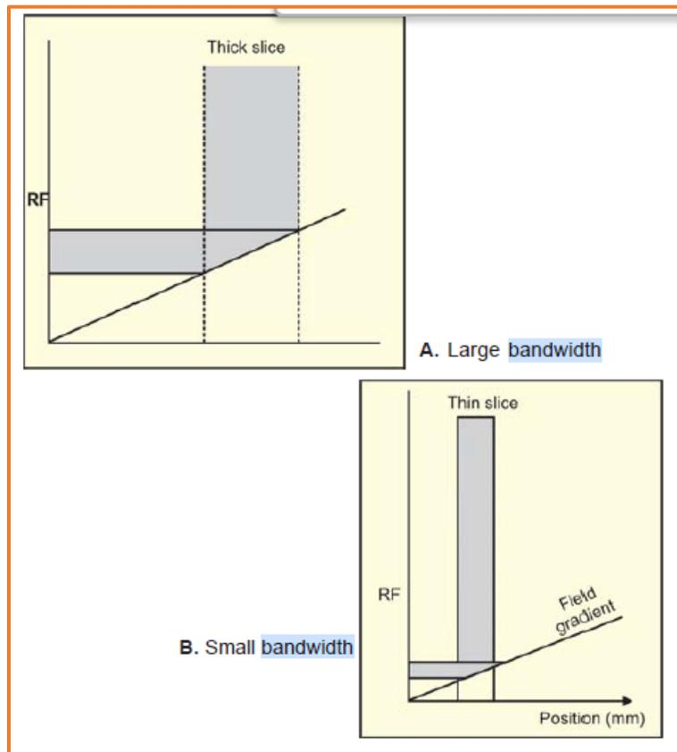
Fig (10 A&B): Selecting slice thickness
