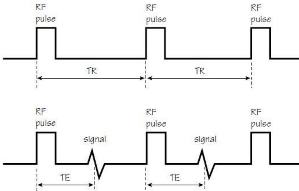
Fig.(2): A basic pulse sequence.
