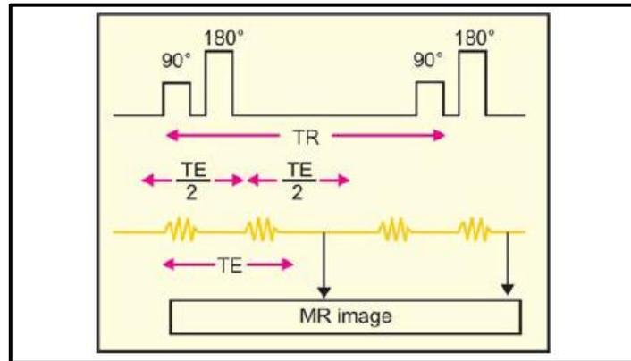
**Fig .(1): Schematic illustration of spin echo pulse sequence**
