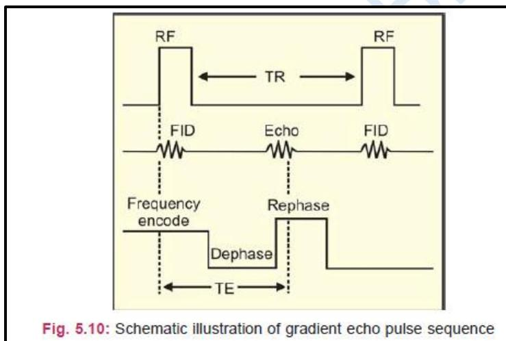
Fig.(8): schematic illustration of gradient echo pulse sequences.
