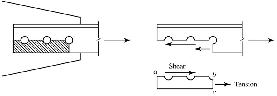
For the case illustrated, the shaded block would tend to fail by shear along the longitudinal section  $ab$  and by tension on the transverse section  $bc$ .
