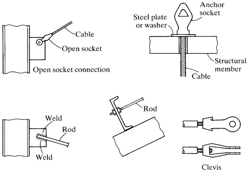
The effective cross-sectional area in the threaded portion of a rod is called the *stress area* and is a function of the unthreaded diameter and the number of threads per inch. The ratio of stress area to nominal area varies but has a lower bound of approximately 0.75. The nominal tensile strength of the threaded rod can therefore be written as
