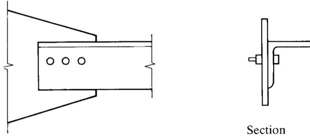
suggests that shear lag be accounted for by using a reduced, or effective, net area. Because shear lag affects both bolted and welded connections, the effective net area concept applies to both types of connections.
