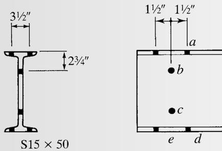
Starting at  $a$  and treating the holes at  $b$  and  $d$  as the staggered holes gives
