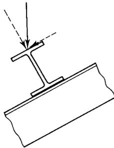
to this type of bending (most shapes used for purlins are very weak in this respect), and the amount of support furnished by the roofing. If a metal deck is used, it will usually be rigidly attached to the purlins, and sag rods may not be needed. Sometimes, however, the weight of the purlin itself is enough to cause problems, and sag rods may be needed to provide support during construction before the deck is in place.
