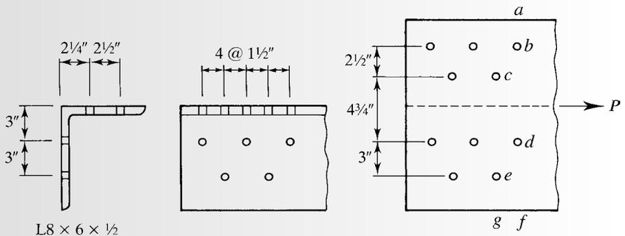
of  $5.413 \text{ in.}^2$  should be multiplied by  $^{10}/_9$  to obtain a net area that can be compared with those lines that resist the full load. Use  $A_n = 5.413(^{10}/_9) = 6.014 \text{ in.}^2$  For line *abcdeg*,
