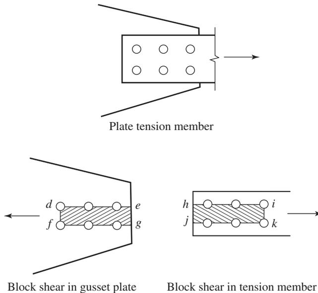
stress, so the nominal strength in shear is  $0.6F_uA_{nv}$  and the nominal strength in tension is  $F_uA_{nt}$ ,
