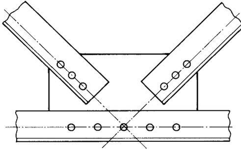
The fact that chord members are continuous and joints are bolted or welded would seem to invalidate the usual assumption that the truss is pin-connected. Joint rigidity does introduce some bending moment into the members, but it is usually small and considered to be a secondary effect. The usual practice is to ignore it. Bending caused by loads directly applied to members between the joints, however, must be taken into account. We consider this condition in Chapter 6, “Beam–Columns.”
