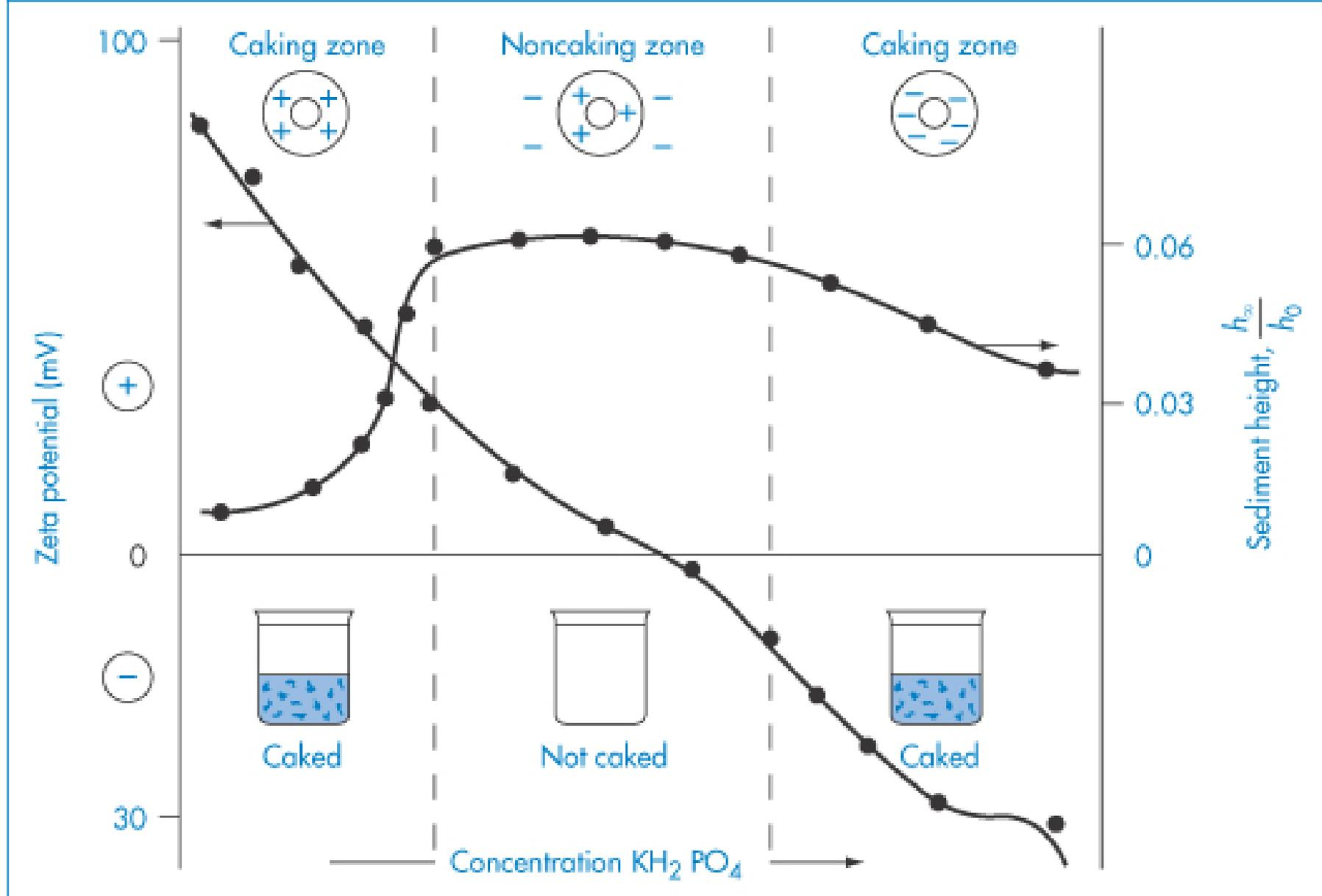
**Caking diagram, showing the flocculation of suspension by means of the electrolyte**
