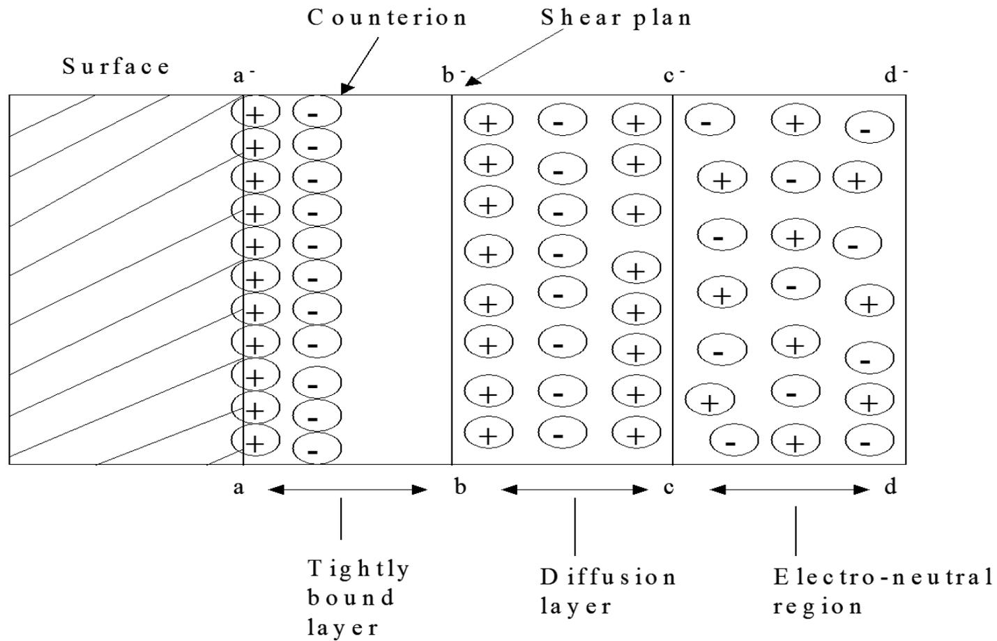
**Zeta potential** is the *potential difference* between the ions in the tightly bound layer and the electroneutral region.
