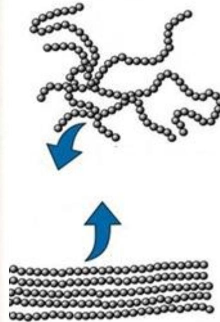
Entangled structure of polymer chain at rest
