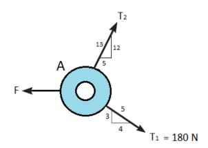
**Example No. 2:** The 290 N pipe is supported at A by a system of five-cords. Determine the force in each cord for equilibrium.
