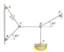
**Answer**:  $T_{DE} = 392.4 N$ ,  $T_{CD} = 339.83 N$ ,  $T_{CB} = 274.62 N$ ,  $T_{CA} = 242.73 N$
