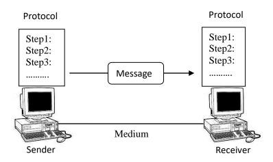
Figure (1) Components of a Data Communication System
