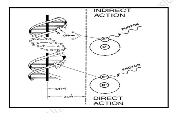
Mechanisms of Radiation Damage
