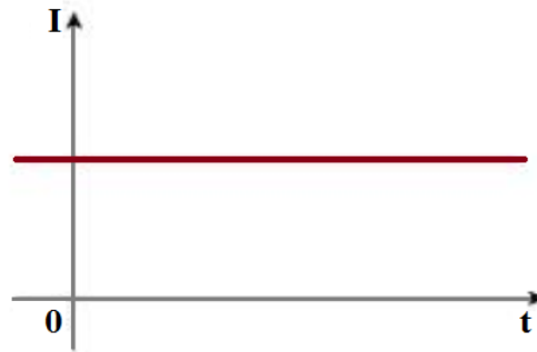
Fig.(7) Direct current (dc), constant with time.
