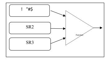
The theory is that addition with carry destroys the algebraic properties of LFSRs, and that XOR destroys the algebraic properties of FCSRs. This generator combines those ideas, as used in the LFSR/FCSR Summation Generator and the LFSR/FCSR Parity Generator just listed, with the Gollmann cascade.
