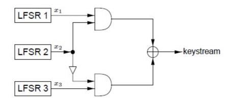
(Hardmard Generator) :Nonlinear generator consists of two LFSR of (X1,X2) with nonlinear function
