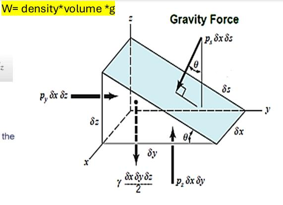
• The equations of motion (Newton's second law, F m a in the y and z directions are, respectively, Force balance
