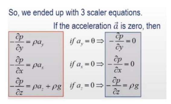
Hydrostatic Condition(a = 0)
