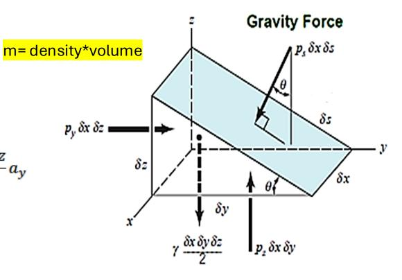
• The equations of motion (Newton's second law, F m a in the y and z directions are, respectively, Force balance
