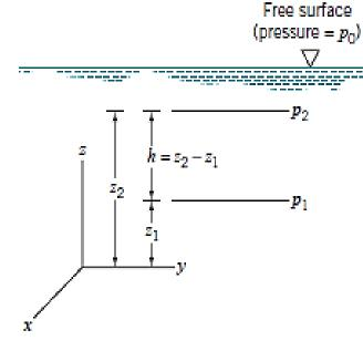
This type of pressure distribution is commonly called a hydrostatic distribution
