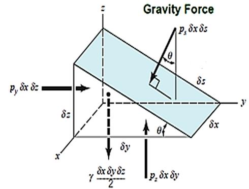
Pascal's Law the pressure at a point in a fluid at rest, or in motion, is independent of the direction as long as there are no shearing stresses present
