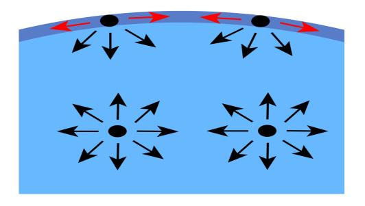
**Due to** the cohesive forces, a molecule located away from the surface is pulled equally in every direction by neighboring liquid molecules, resulting in a net force of zero. The molecules at the surface do not have the *same* molecules on
