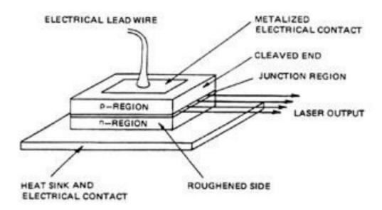
Fig.(11): Basic Semiconductor Laser Design
