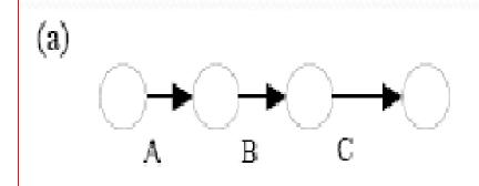
Activity B can be performed only after completing activity A, and activity C can be performed only after completing activity B.
