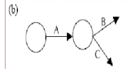
Activities B and C can start simultaneously only after completing A.
