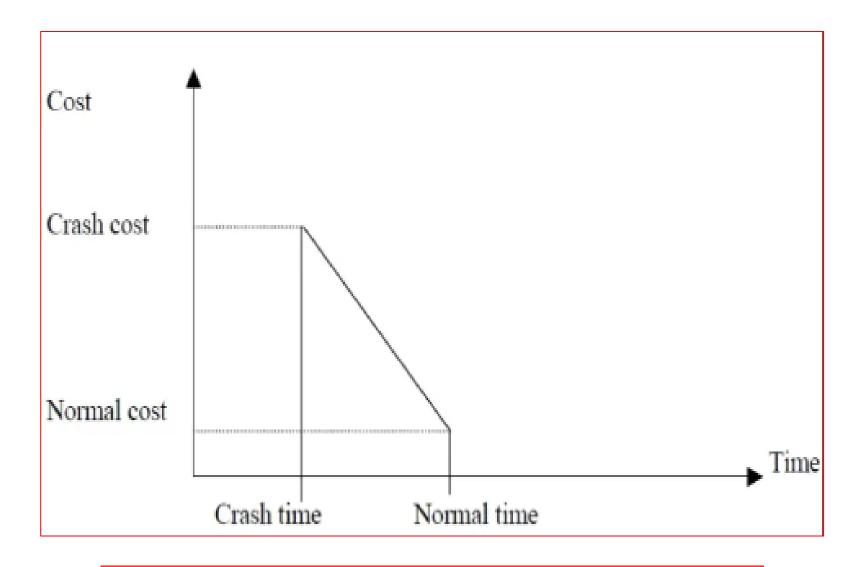
$$Cost \, Slope = \frac{Crash \, Cost - Normal \, Cost}{Normal \, Time - Crash \, Time} = \frac{C_c - N_c}{N_t - C_t}$$
