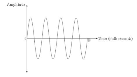
This representation is not always the best representation of the signal for most signal processing related applications. In many cases, the most distinguished information is hidden in the frequency content of the signal. The frequency SPECTRUM of a signal is basically the frequency components of that signal. The frequency spectrum of a signal shows what frequencies exist in the signal. The below represents a signal in time domain and frequency domain.
