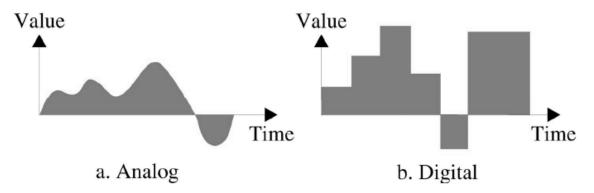
Analog signals are those which are naturally occurring. Any analog signal can be converted to a digital signal. How?
