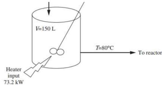
Energy balance at unsteady state around heating vessel
