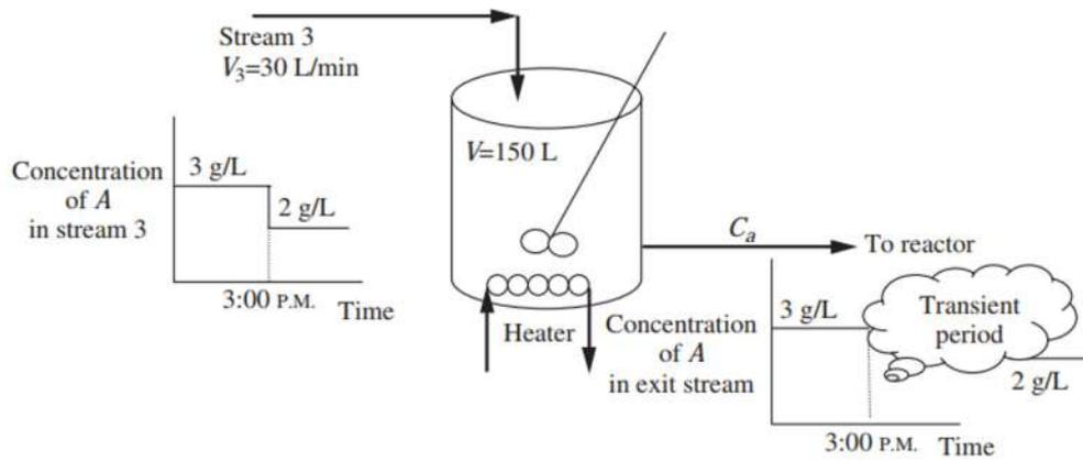
Mass balance on component A around heating vessel at unsteady state
