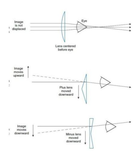
When a lens is decentered, a prismatic effect is created. With decentration, both prism power and prism base direction are manifested.
