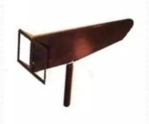
**8.DIPLOSCOPE** - This instrument is based on dissociation of real space.
