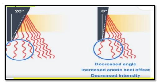
The relationship between anode angle and heel effect in inverse, meaning as the anode angle decreases the anode heel effect increases. (increased difference in the intensity across the x-ray beam
