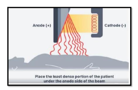
A few variables can actually change the extent of the anode heel effect. -In other words, the change in beam intensity across the beam isn't always the same. Decreasing the anode angle (making it steeper or smaller) increases the anode heel effect
