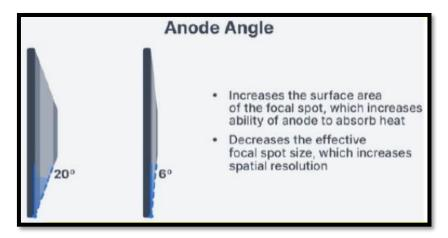
The angled anode does have one negative consequence. The angle of the anode does cause a variation of the beams **intensity** across the x-ray field. Specifically,
