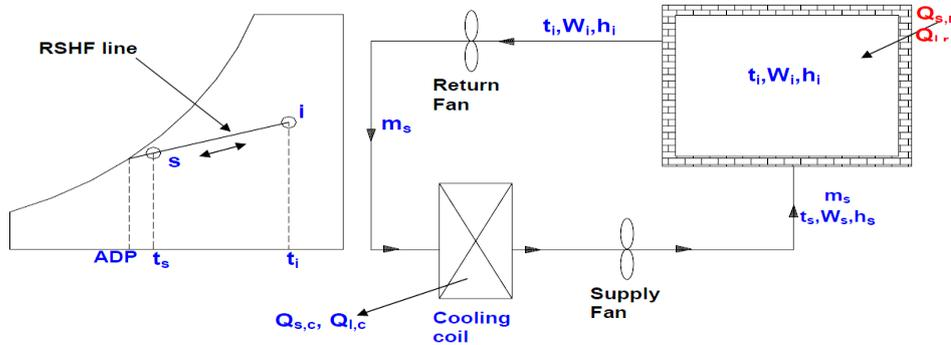
**Fig.1: A summer air conditioning system with 100% re-circulated air**
