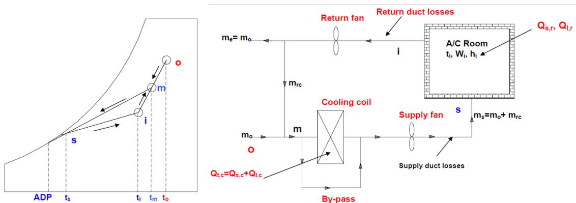
**Fig.3: A summer air conditioning system with outdoor air for ventilation with by-pass factors**
