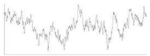
The above waveform does not have fixed number of voltage values (i.e unlimited or  $\infty$ ). In this case we can not define certain probability of such voltage. Instead, we may talk about range of voltage, maximum, minimum, average....etc.
