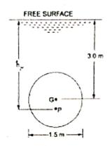
$$\begin{split} A &= \frac{\pi}{4} \times (\ 1.5\ )^2 = 1.767\ m^2 \quad ,\ h_c = 3\ m \\ F &= \rho\ g\ A\ h_c = 1000 \times 9.81 \times 1.767 \times 3 = 52002.81\ N \\ h_p &= \frac{I_G}{Ah_c} +\ h_c \quad ,\ I_G = \frac{\pi\ d^4}{64} = \frac{\pi\ (1.5)^4}{64} = 0.2485\ m^4 \\ h_p &= \frac{0.2485}{1.767 \times 3} \ +\ 3 = 0.0468\ + 3 = 3.0468\ m \end{split}$$
