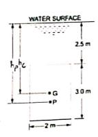
$$h_c = 2.5 + \frac{3}{2} = 4 \text{ m}, F = \rho \text{ g A } h_c = 1000 \times 9.81 \times 6 \times 4 = 235440 \text{ N}$$
