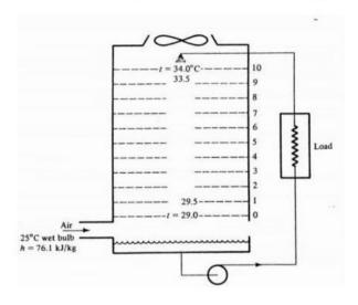
19-3 Analysis of a counterflow cooling tower One design of cooling tower is the counterflow type, in which air passes upward through a falling spray of water. Figure 19-3 shows a differential volume of a counterflow cooling tower with L kg/s of water entering from the top and G kg/s of air entering from the bottom. For simplicity, the small quantity of water which evaporates is neglected, so that both L and G remain constant throughout the tower.
