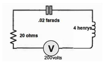
Based on the diagram above, our circuit has an inductor of 4 henrys, a resistor of 20 ohms and a capacitor of .02 farads. As for the charge and current, let's set a condition so that the charge on the capacitor, and current in the circuit, be 0 at t=0. Let's find the charge on the capacitor at any time t besides 0, where V is equal to 200 volts. So then we get the following,
