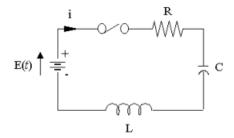
**Example:** An inductance of  $\overline{3}$  henry, a resistor of 16 ohms and a capacitor of 0.02 farad are connected in series with an emf of 300 volts. At t=0, the charge on the capacitor and current in the circuit is zero. Find the charge and current at any time t>0.
