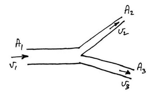
**Example:** The diameters of a pipe at the sections 1 and 2 are 10cm and 15cm respectively. Find the discharge through the pipe if the velocity of water flowing through the pipe at section 1 is 5m/s. Determine the velocity at section 2.
